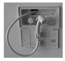
The exterior wash station is located on the roadside or rear of the trailer. It provides both hot and cold water. It uses water from the fresh water tank or when connected to the city water hookup. The showerhead is equipped with a flow control to allow you to conserve water. The flow control is not a permanent shut off. After use, the water must be shut off at the control valves.
