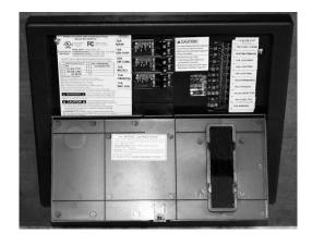
A 12-volt interior fuse panel is installed in the Power Distribution Center to protect the interior circuits. Circuit titles and fuse sizes are marked inside the access door. If a fuse blows, locate and correct the cause. Turn off all lights and motors, and then install a fuse with the same rating. If fuses continue to blow, a short circuit is indicated. Have the system checked by qualified personnel.
