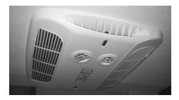
The roof-mounted Air Conditioner operates on 120-volt power, which is supplied through the 30-amp power cord, either from an outside 120-volt power service or by the onboard generator, if equipped.
