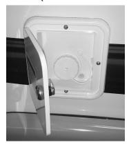
The fresh water system should be sanitized at the initial filling, after a period of storage or if contaminated. See "Sanitize Fresh Water System" in this section. Fill tank slowly. Do not overfill. Do not leave unattended while filling. Structure damage may occur.
