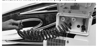
The exterior wash station is located in the docking station located on the roadside for exterior use. It uses water from the fresh water tank or when connected to the city water hookup. The showerhead is equipped with a flow control to allow you to conserve water.
