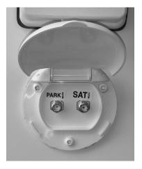
The park/sat dish inlets are located on the driver's side of the trailer. The park cable inlet allows for the connection from the campground cable service to the trailer. The satellite inlet allows for the connection from a portable dish. Both cables terminate inside the camper at the primary TV location in a wall plate. The park cable is connected to the 12-volt/TV outlet. With the switch on the outlet in the "OFF" position, the park cable signal is sent through the outlet.
