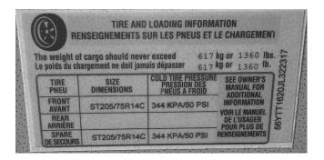
The first (upper) label is the Tire and Loading Information Tag. It lists the trailer VIN number and maximum cargo capacity of the trailer as equipped by Lance. It also lists the tire size and Cold Tire Pressure of the tires that are supplied on your trailer.
