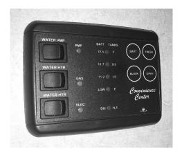
The systems monitor panel incorporates controls for the water and holding tank levels, battery condition and water pump. It may also control the water heater.
