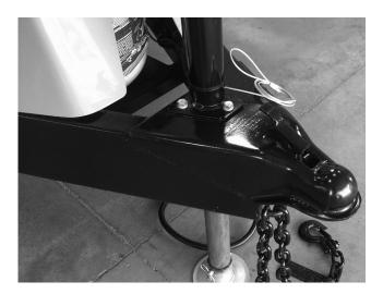
The ball hitch trailer is fitted with a tongue jack that can raise and lower the coupler. The tongue jack is mounted to the A-frame part of the trailer. By rotating the jack handle clockwise, the jack will extend and raise the tongue of the trailer.
