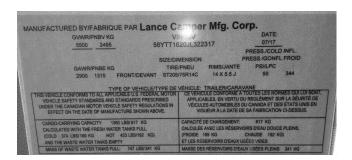
The second (lower) label is the Federal Certification Tag. It contains the Manufacturer's Name, VIN number, month and year built, GVWR, GAWR of each axle, and the tire size, rim size and PSI.
