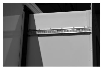
The slide-out room uses an in-wall mechanism to move the room. The mechanism is driven by two (2) 12-volt DC motors by the trailer battery(s). A switch mounted on the wall controls the room movement.
