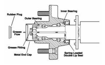
Bearings should be inspected for corrosion or wear, cleaned and re-packed every 12 months or 12,000 miles.
