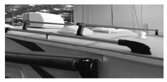
The towers and cross bars are mounted to the roof racks that allow other accessories to be added to accommodate transporting other items on the roof of your trailer. Roof rail capacity with towers and cross bars is 500 lbs. Be sure to spread the load across the rails. Accessories for the crossbars are available from your Lance Dealer or a local sporting goods retailer.
