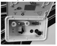
The water tank fill is located in the exterior docking station located on the roadside of your trailer.
