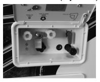
The city water connection is located in the exterior docking station located on the roadside of your trailer.
