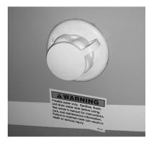
The city water inlet connection is located on the roadside of your trailer.
