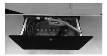
A fuel transfer system allows you to store gasoline for use in motorcycles, snowmobiles, ATVs or other vehicles and equipment while at a campsite. This system consists of a fuel tank, fuel tank filler, fuel gauge, fuel transfer pump, fuel transfer valve and hose with fill nozzle. Your trailer is equipped with a timer switch allowing the pump to run for five minute intervals. To
