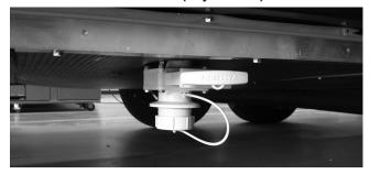
The water system should be drained if it will be out of service for more than one week. This will prevent algae and bacteria contamination of your fresh water system.
